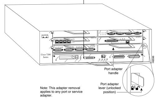
Step 3 Grasp the handle on the port adapter and pull the port adapter from the midplane, about halfway out of its slot. If you are removing a blank port adapter, pull the blank port adapter completely out of the chassis slot.
